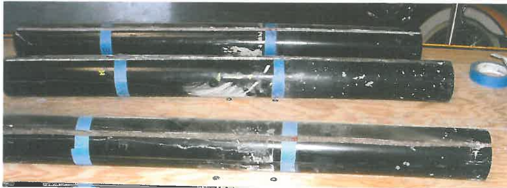
Photo 5b. Pole Sections After Longitudinal Cutting, But Before Opening The Sections.
