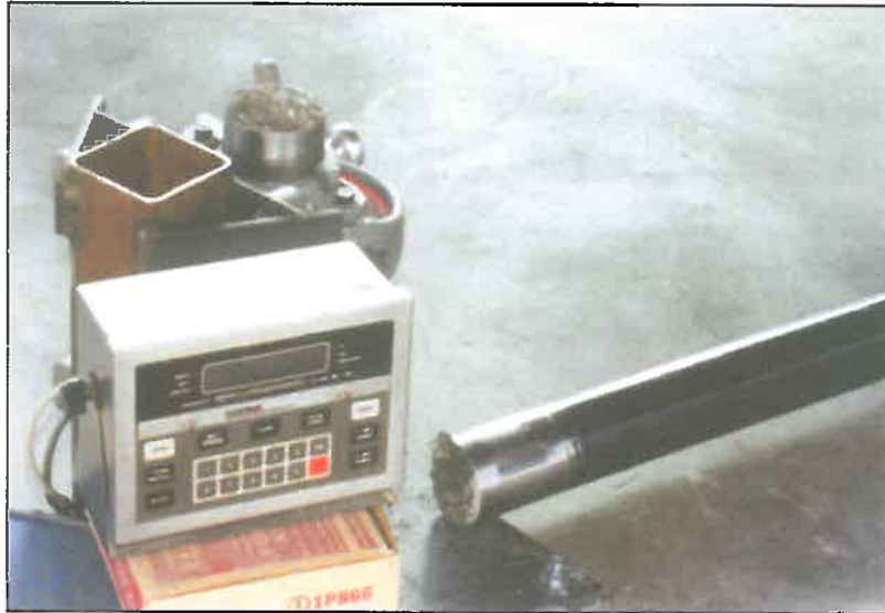
Photo 6b. Machined Exemplar Pole Without Reinforcing Bar In Concrete, After Test.
