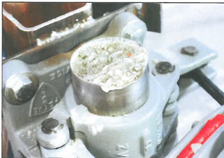
Photo 6c. Close-up Of Failure Of Machined Exemplar Pole
