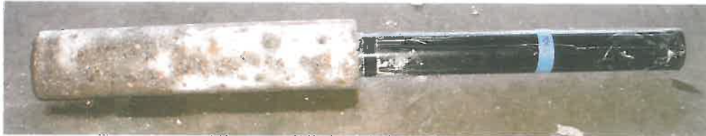
Photo 5a. Pole Section After Vibration, And Removal From Concrete Base.
